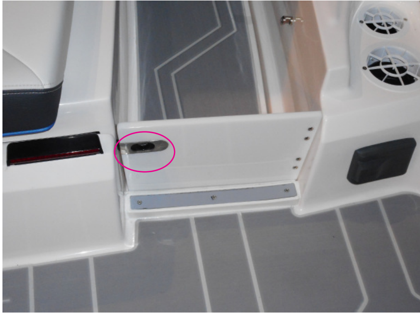
Typical Transom Door (Gate) Showing Latch
