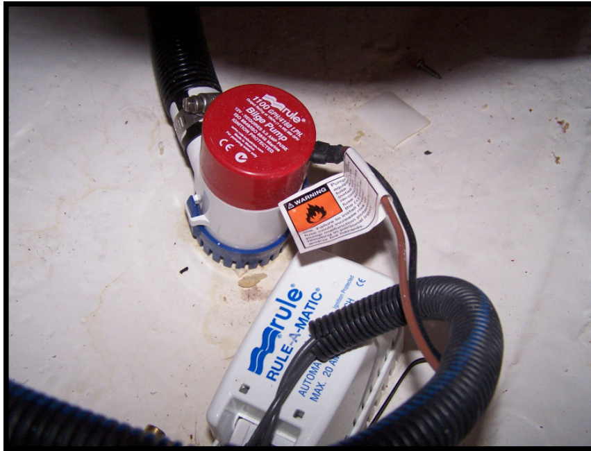
Typical Bilge Pump And Automatic Float Switch
