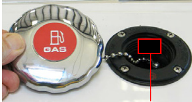
COMBO FUEL FILL W/ INTERNAL VENT
