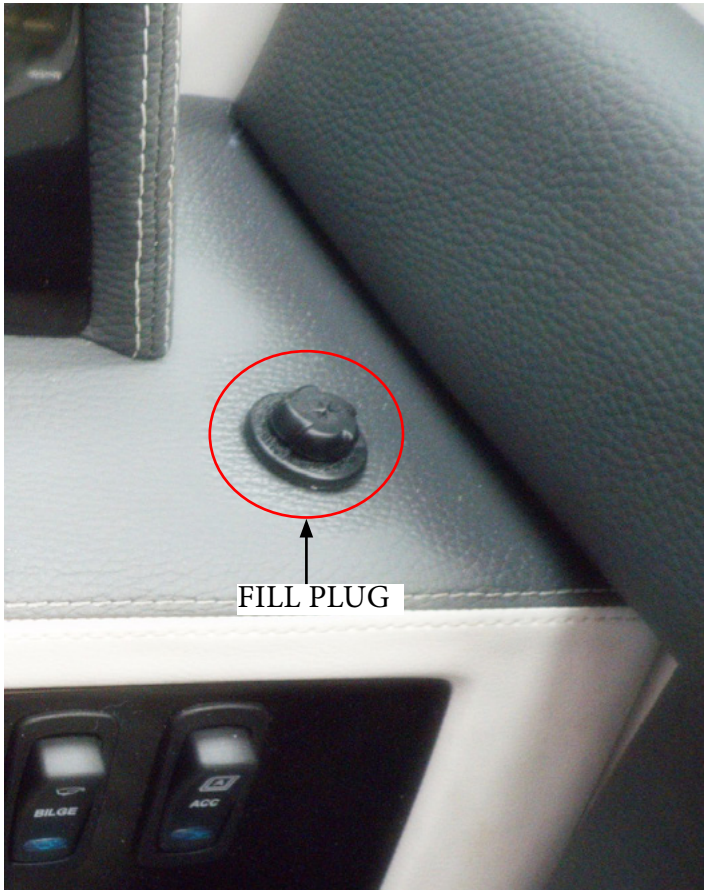
FILLING HELM HYDRAULIC STEERING FLUID
