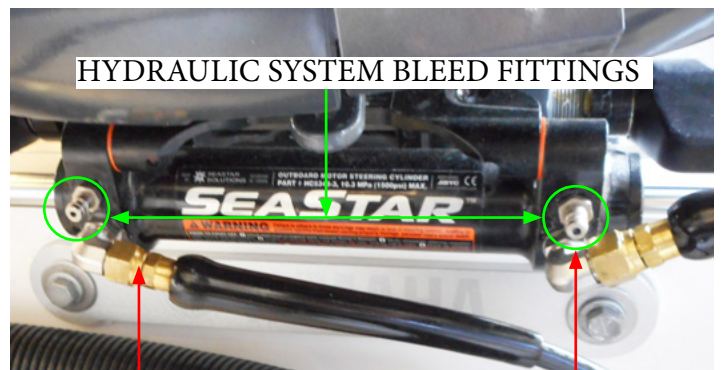
STEERING HARDWARE & HOSES AT ENGINE
