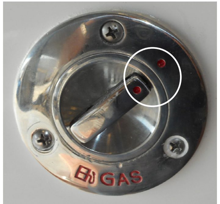
FUEL FILL CLOSED AND POINTS LINED UP
