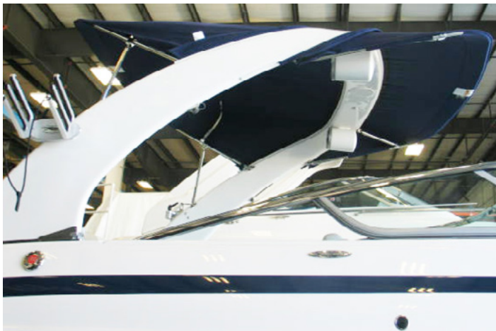
TYPICAL POWER TOWER- SUNSHADES IN CRUISE POSITION
