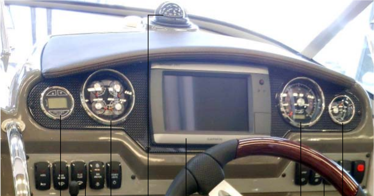
Depth Gauge Multi-Gauge Optional Chartplotter Tachometer Trim Gauge Port Switch Panel Compass Stbd. Switch Panel
