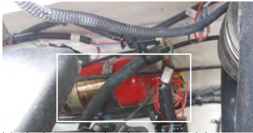
Typical Automatic Fire Extinguisher Canister Location
