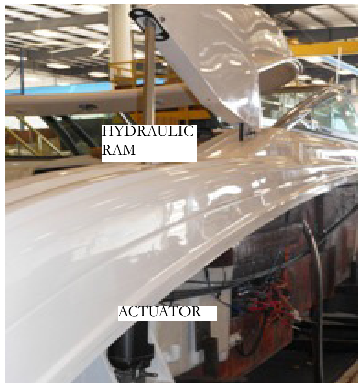
TYPICAL POWER TOWER IN FWD. POSITION
