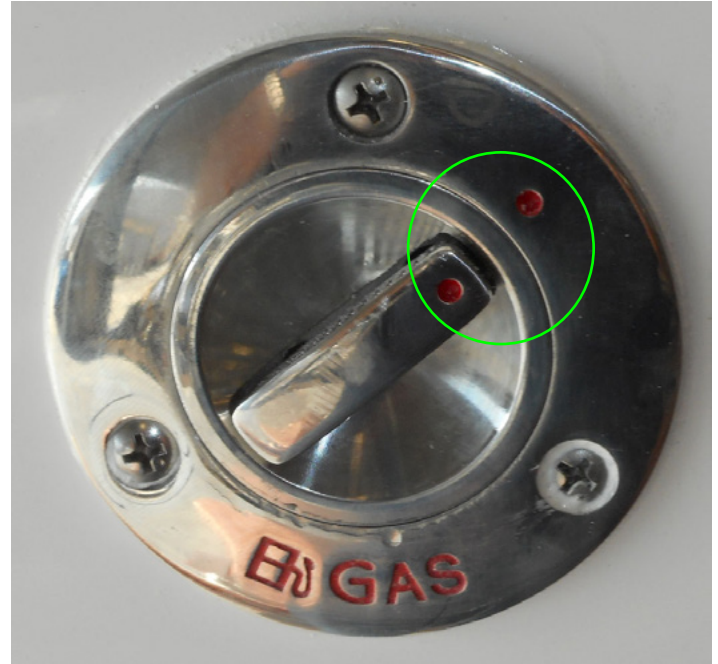
FUEL FILL CLOSED AND POINTS LINED UP
