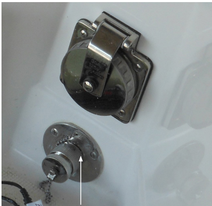
TYPICAL DOCKSIDE WATER INLET
