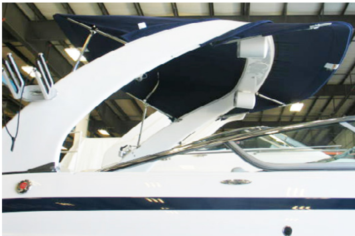
TYPICAL POWER TOWER- SUNSHADES IN CRUISE POSITION
