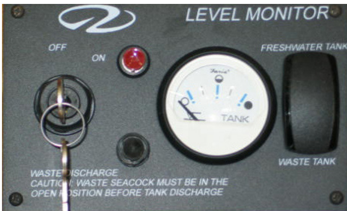
TYPICAL WATER/WASTE MONITOR PANEL
