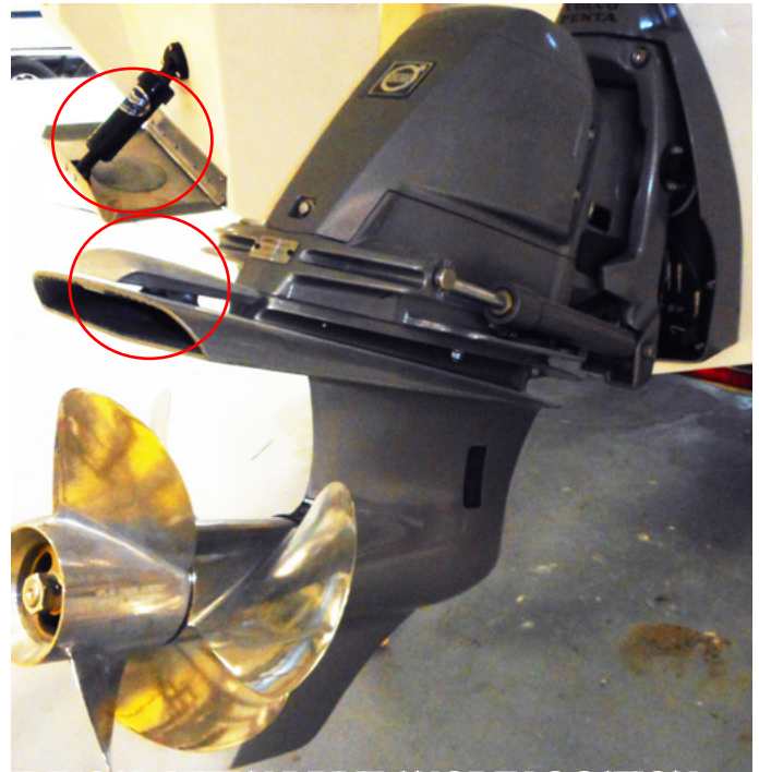
TYPICAL STERN DRIVE ANODE LOCATION
