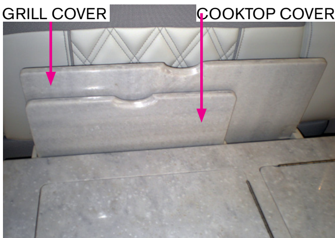
COOKTOP COVERS IN PROPER SLOTS FOR ACTIVATING CONTROL PANELS
