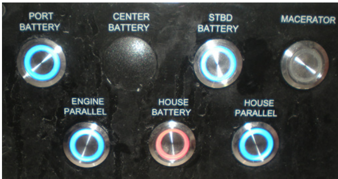
TYPICAL EARLIER BATTERY ACTIVATION PANEL
