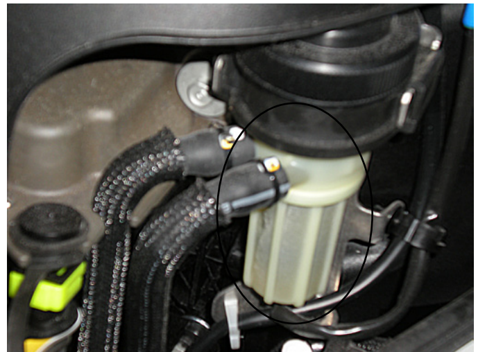
FUEL FILTER ELEMENT INSIDE FILTER BODY
