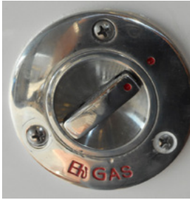
COMBO FUEL FILL/ INTERNAL VENT
