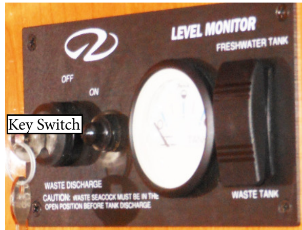
FRESH WATER & WASTE MONITOR WITH OVERBOARD DISCHARGE
