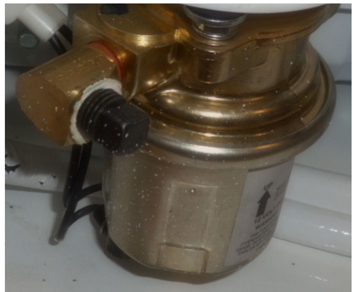
TYPICAL GENERATOR INTEGRATED FUEL FILTER
