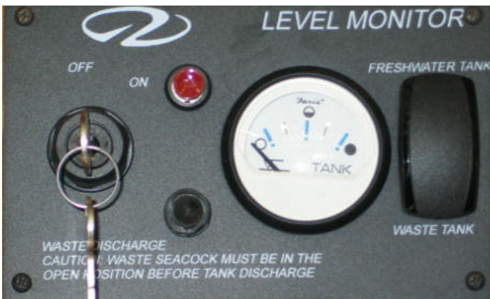
TYPICAL WATER/WASTE MONITOR PANEL
