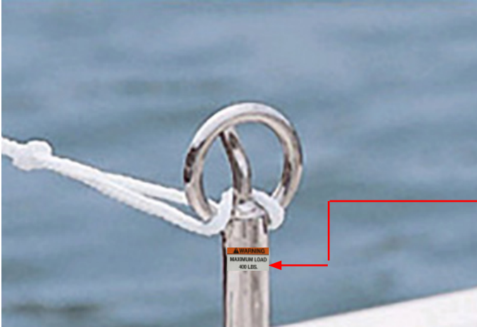
TYPICAL WATER SPORTS OUTBOARD PYLON
