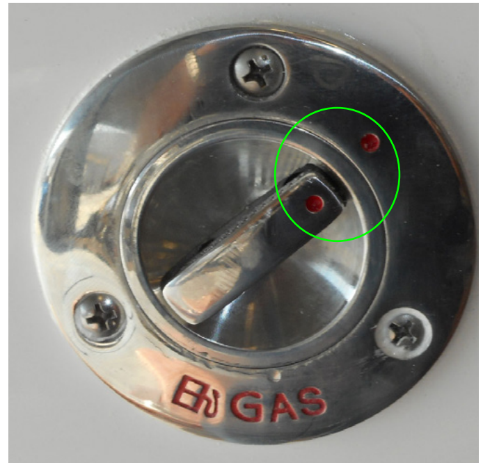
FUEL FILL CLOSED AND POINTS LINED UP
