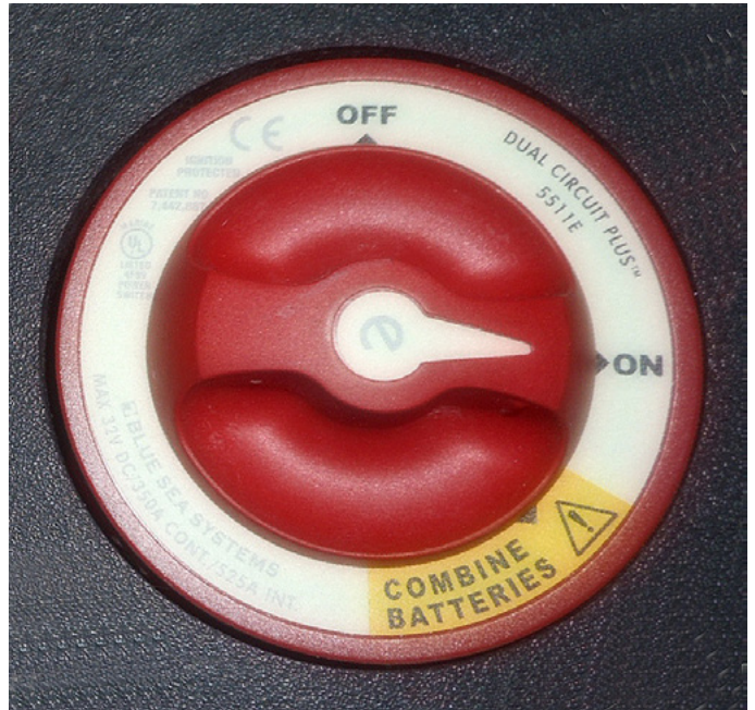
TYPICAL DUAL BATTERY SWITCH
