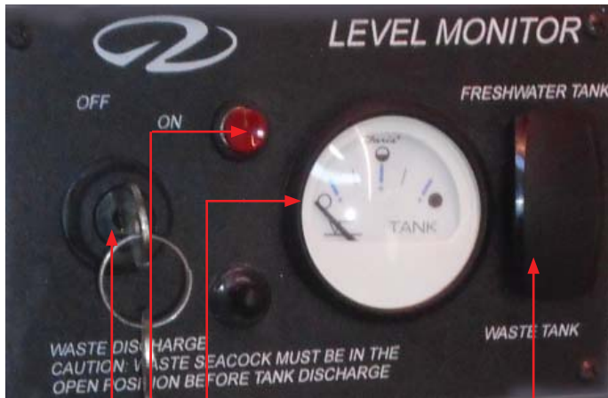
KEY GAUGE MOMENTARY SWITCH PUMP-OUT BUTTON
