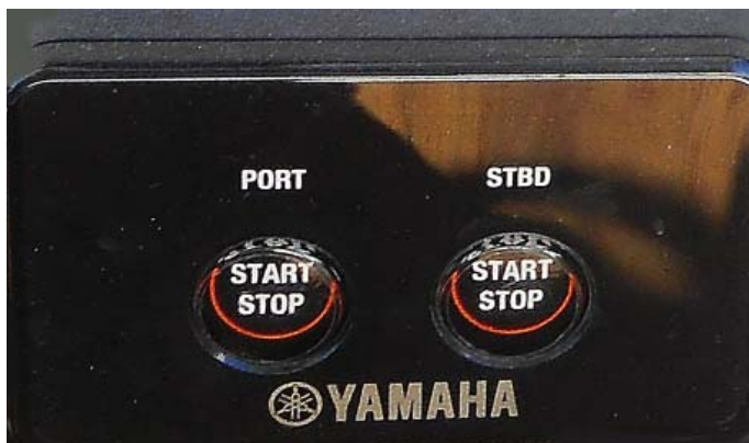
Typical Start/Stop Panel
