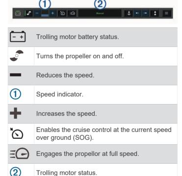
Enables anchor lock, which uses the trolling
