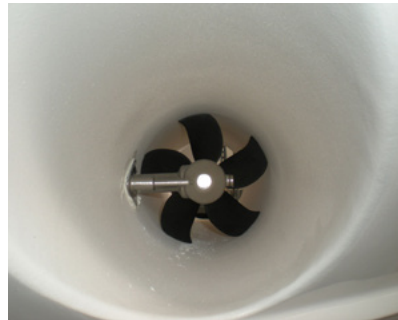
THRUSTER PROP AT HULL
