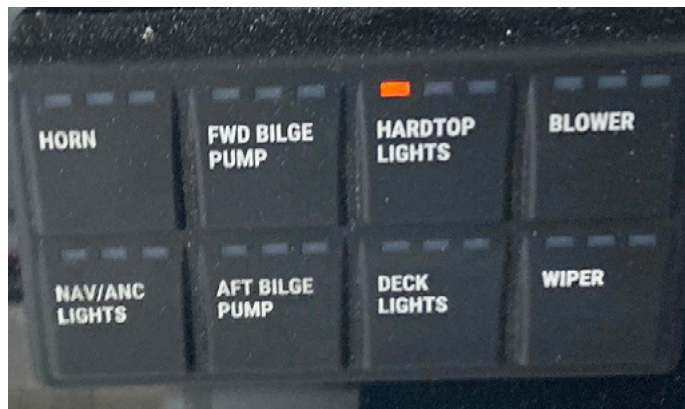
TYPICAL WIPER FUNCTION- SWITCH PANEL
