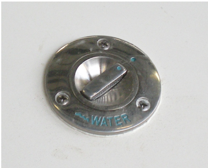
FRESH WATER FILL- TYPICAL DECK FITTING
