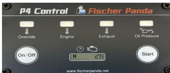
FISCHER PANDA P4 GEN CONTROL PANEL
