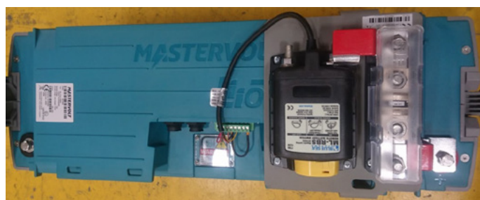
TYPICAL LITHIUM-ION BATTERY
