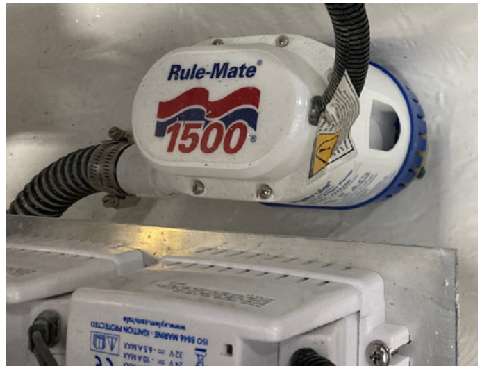
Typical Bilge Pump And Automatic Switch
